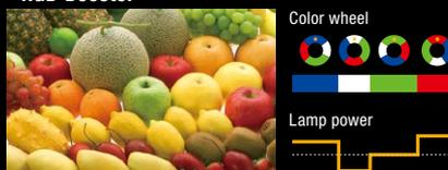
By modulating the lamp power, we can maximize the color reproduction of each color without sacrificing brightness. Light usage is optimized, and color balance is obtained without lowering the brightness.
